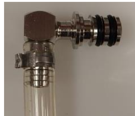
QD Connector Kit for Sweetener Line (Coca-Cola Part # TBD)
